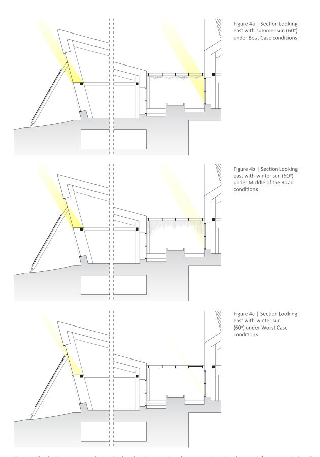
Figure 4. The shading system was designed to be adaptable to various climate scenarios using the same infrastructure in the adjustable PV panels and vegetated trellis that could accommodate a fixed panel if necessary.
