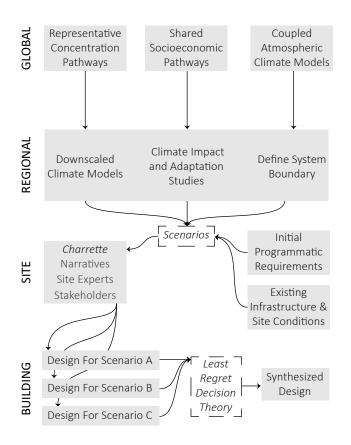
Figure 2. The framework for the project operated across four scales with each step in the design process focusing in closer to the building.
